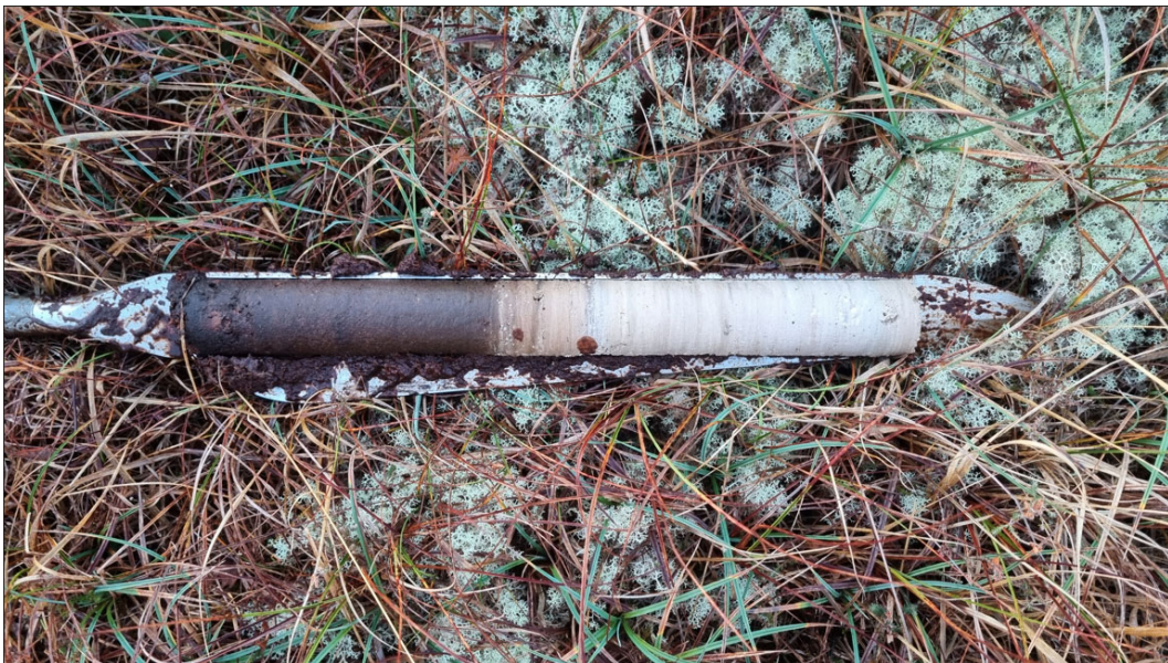
Figure 2.4: RS_01 – The base of peat was encountered at 3.20 m bgl, underlain by soft white shell marl.
