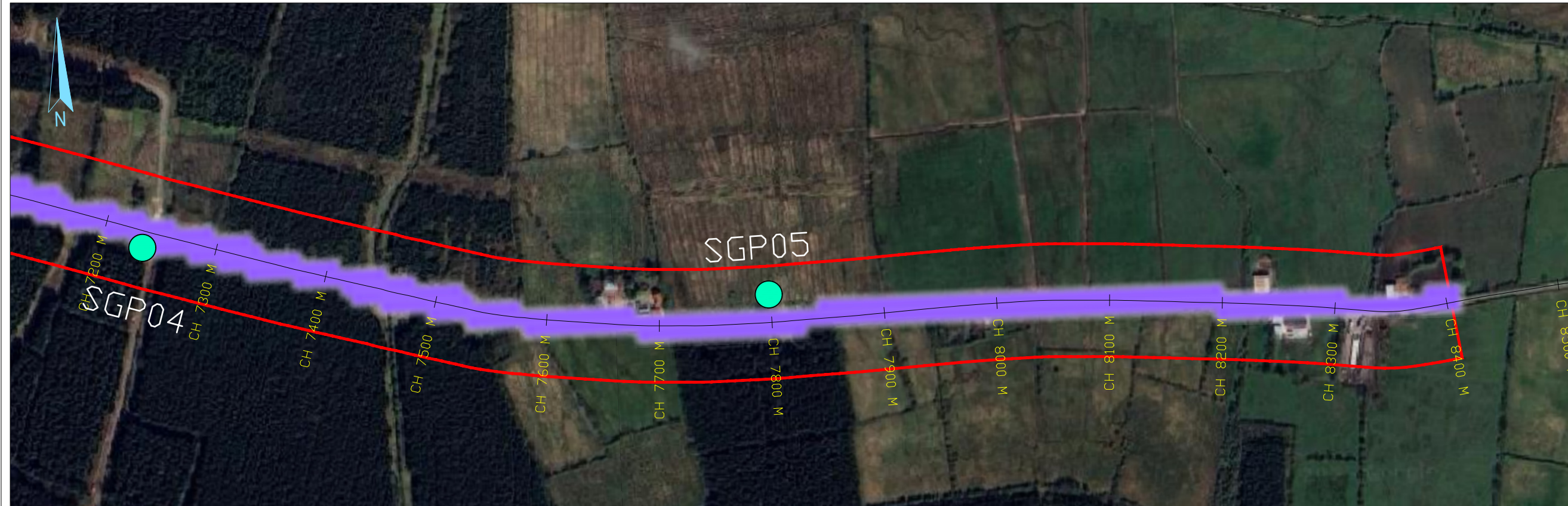
FIGURE 2: GPR SECTION 1 (CHAINAGE: 7200 - 8410 m) - GPR INTERPRETATION - FLAT DATUM
